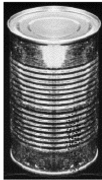
Pitted rust or leaking
